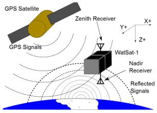
Figure 1: WatSat-1 Antenna Orientation
